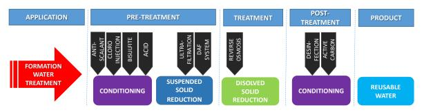
Complete flowchart for formation water reuse below showing the ADVANCEES systems. This flowchart vary based on raw water quality and customer's requirement. Many options and combinations are possible, the best solution needs to accommodate the minimum life cycle cost such as low operating cost, low maintenance, easy to operate and monitor
